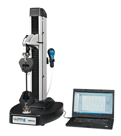
The LS1 is a 1 kN / 225 lbf high precision material testing machine that combined with our extensive range of grips, fixtures, extensometers and software creates a powerful material testing system. The system is equally suited to quality control, educational and R&D environments within a wide range of applications and test types, including medical devices, plastics, packaging, textiles, rubber and electronics to name a few.
